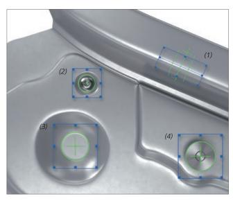
One benefit of dense point clouds is that multiple features, such as bending edges, rivets, surfaces points and T pins, can be measured with just a single capture.
