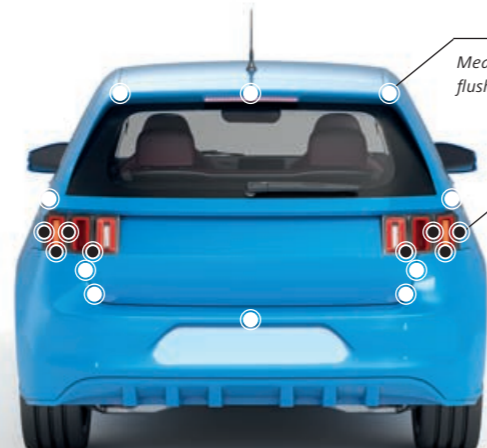
Measurement of flush and gap on headlamps
